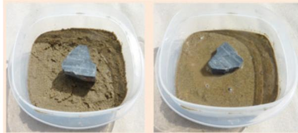
**Figure 12.28** Fine, damp sand before shaking (left) and after (right). *Source: Steven Earle (2015) CC BY 4.0*
