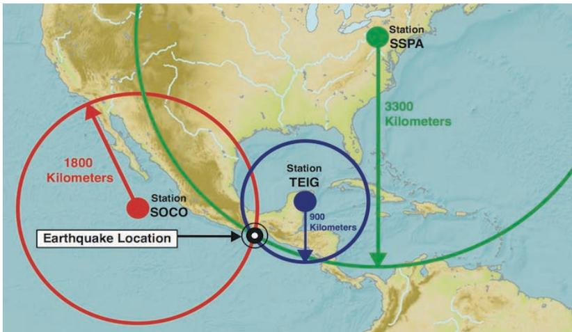
**Figure 12.12** Locating earthquakes by drawing three circles with radii of lengths determined from P-wave and S-wave travel times. Station names (SOCO, TEIG, SSPA) correspond to seismograms in Figure 12.11. *Source: IRIS (n.d.) "How Are Earthquakes Located?" See Appendix C for terms of use.*
