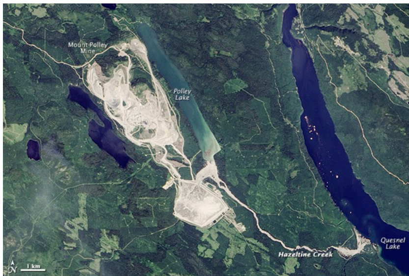
Figure 18.14b The Mt. Polley Mine area after the tailings dam breach of August 2014. The water and tailings released flowed into Hazeltine Creek, and Polley and Quesnel Lakes. [ https://en.wikipedia.org/wiki/Mount_Polley_mine_disaster ] ]
